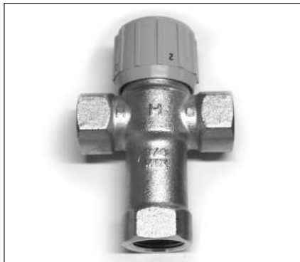
Figure 20 - Adjust Thermostatic Mixing Valves at each point-of-use to 120°F (49°C) or lower.
