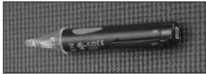
Figure 21 - Use a non-contact circuit tester to check for electrical power.
