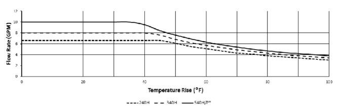
\*Maximum flow rate with set temperature above 130°F (55°C) is 8.0 GPM.
