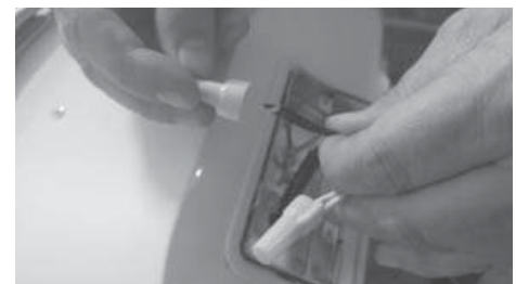
Figure 18 - Connecting the electrical wires.
