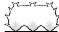
UNSTABLE YELLOW FLAMES • Unstable flames; no defined cones • Hazy, yellow flame • Correct by rotating air shutter clockwise ↷.
